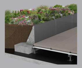
This is where a concrete foundation is cast to the perimeter of the planter, the panels and components are bolted together and mechanically fixed to this foundation.
