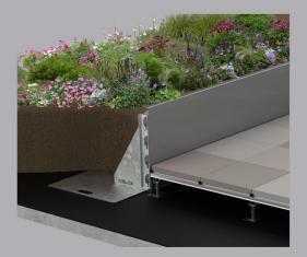
This system utilises the weight of the soil within the planter to provide stability via base plates connected to the planter panels. As a result, no concrete foundation is required, likewise no mechanical fixings. For more information refer to the Velox Rapid Edge system datasheet or contact the Logic technical team.
