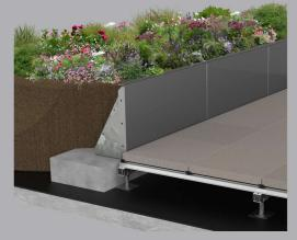
This is where a concrete foundation is cast to the perimeter of the planter, the panels and components are bolted together and mechanically fixed to this foundation. The foundation provides stability and lateral support to the edge.
