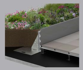
This design has an elevated platform, usually provided by a pedestal-n-rail system, which the planter edge is then secured to. Metal plates (sometimes paving) are extended beneath the planter which provide the base and fixing point for the raised edge.
